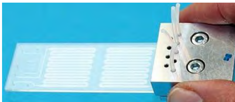
Figure 1 Chip device with droplet generator and incubation channel.
